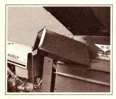
Optional center shaft feed opening\*, available on the 5-20-VL, lets you direct limbs and branches up to 3" in diameter directly into the center of a heavy-duty cylinder.
